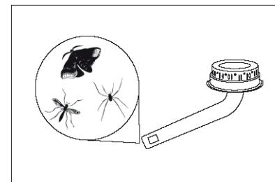
This may prevent gas from arriving to the venturi tube, causing yellowish, smoky flame at the burner or rendering lighting of the burner impossible. This could even result in combustion of the gas outside the supply tube, which may seriously damage the barbecue.
